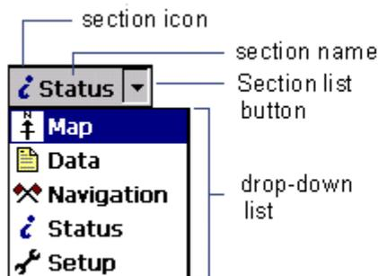
One of these sections is always active and visible. The Section list button shows the section that is currently active. You can move between sections at any time without closing any open forms or screens. To switch to a different section, tap the Section list button and then select the section you want from the drop-down list.
