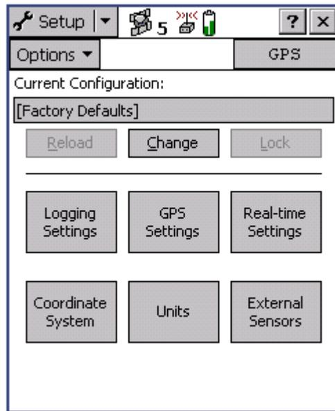
From the previous section - if the satellite icon on the top of the screen is not in view. Tap **GPS** or from the Options submenu, choose **Connect to GPS**
