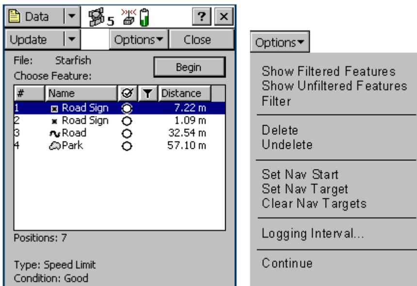
Once a Nav Target is selected, switch to the NAV screen by selecting **Navigation** from the **Section** List
