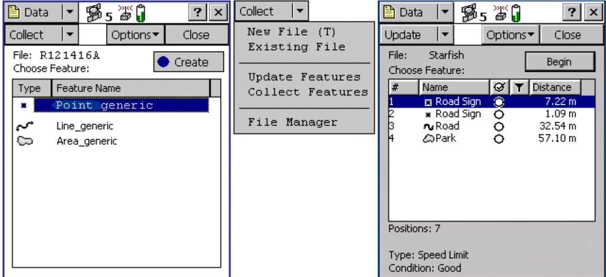
In order to Navigate to a point, It must first be selected. **Set Nav Target** may be selected from the: **Data Update** screen by highlighting the desired point then from the **Options** Tab, select **Set Nav Target**. Or from the;
