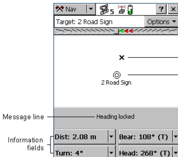
When within the specified Close-up Range of the target, the navigation proximity alarm sounds, and the Close-up graphical screen replaces the Direction Dial screen.
